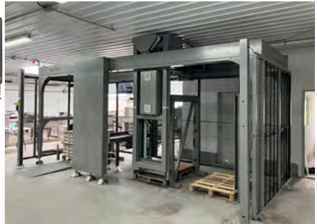
Prinzen Speedpack - 220 Cases Per Hour - 80,000 Eggs Per Hour Fully Automated Egg Palletizing
