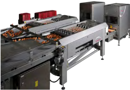
Prinzen Speedpack - 220 Cases Per Hour - 80,000 Eggs Per Hour Fully Automated Egg Palletizing
